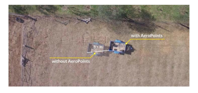
But if you're using a different workflow, like <u>Propeller PPK</u>, the need for traditional ground control is significantly reduced. The Propeller PPK solution uses a Phantom 4 RTK drone and a single AeroPoint as a passive base station.
