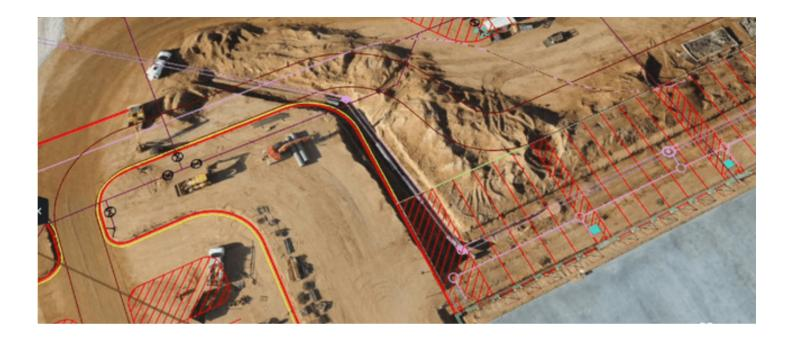
Armed with this information, the team showed how the subcontractors were off in their conduit placement, proving they needed to correct the work or update the model to reflect as-built conditions.
