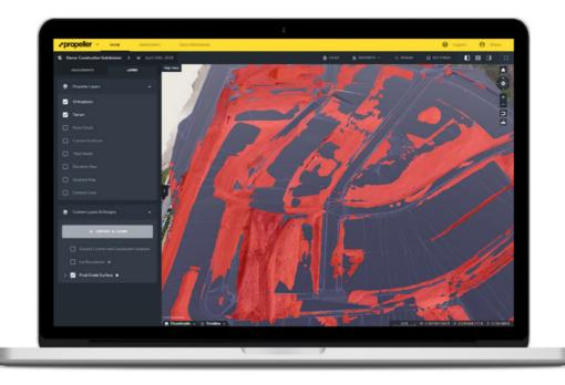
In Propeller, adding designs—whether as linework or design surfaces—allows you to visually monitor and track progress towards that final design. Because the model is 3D and uses up-to-date photographs, it's easy to recognize how the design relates to the current state of your site.
